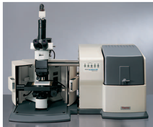
Figure 1: Nicolet Almea XR Dispersive Raman Spectrometer with long working distance objectives, high resolution automated microscope stage, and well plate adapter
