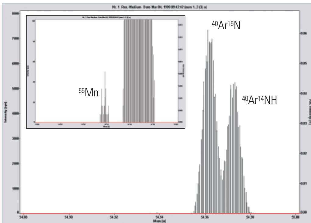
Figure 3: Medium resolution ( $R = 4000$ ) spectrum of manganese ( $m/z$  55) showing  $^{40}\text{Ar}^{15}\text{N}$  and  $^{40}\text{Ar}^{14}\text{NH}$  interferences generated by the TMAH matrix.
