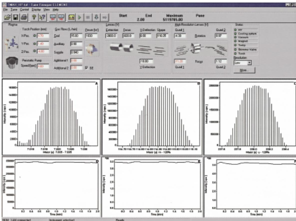
Figure 2: Instrumental sensitivity under hot plasma operating conditions for 0.3 N TMAH solution spiked with 100 pg/g of a multi-elemental solution containing Li, In and U.
