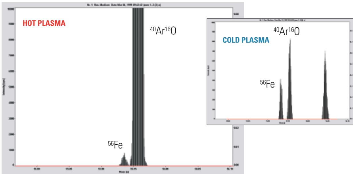
Figure 4: Medium resolution ( $R = 4000$ ) of iron ( $m/z$  56) showing the difference polyatomic interferences observed under hot and cold plasma conditions.
